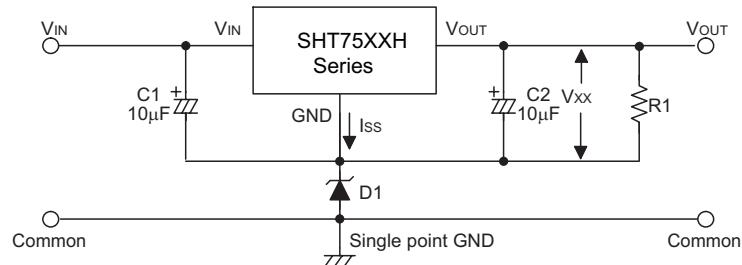
$$V_{OUT} = V_{xx} + V_{D1}$$
