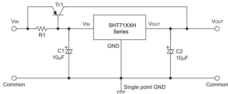
**Short-Circuit Protection by Tr1**
