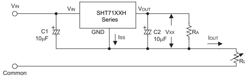
$$I_{OUT} = \frac{V_{xx}}{R_A} + I_{ss}$$
