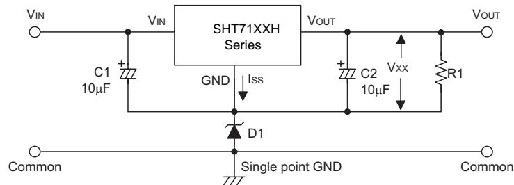
$$V_{OUT} = V_{xx} + V_{D1}$$
