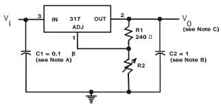
Note A: Use of an input bypass capacitor is recommended if regulator is far from filter capacitors. Note B: Use of an output capacitor improves transient response but is optional.
