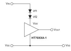
Detectable Voltage =  $V_{f1}+V_{f2}+V_{DET}$
