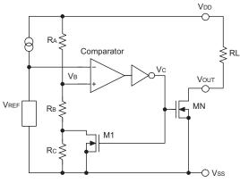
NMOS Output Voltage Detector (HT70XXA-1)
