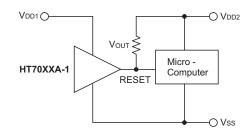
• NMOS open drain output application with R-C delay
